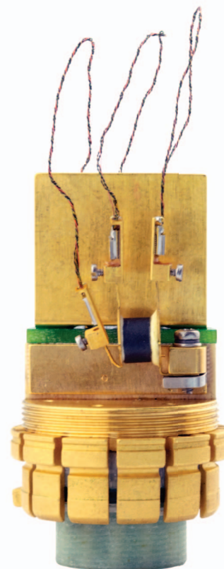
TTO Puck with Disk-Shaped Sample Installed
