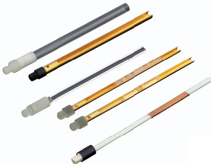
Various sample holders for VSM measurements. The straw holder (top) and large brass trough are only compatible with the LBC, whereas the quartz paddle, small brass trough (with polycarbonate powder holders) and quartz bracers (shown), and heater stick (for VSM Oven measurements) can all be used with the standard bore coil set.
